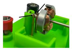
Push the Magnet Bar (B) on the Plastic Base (A) where the rectangular supports are. Connect battery holder (with AA battery) to the Coil Terminals (C, D). The motor should start spinning. If not, try spinning the Armature Shaft (G) to start the motor.
